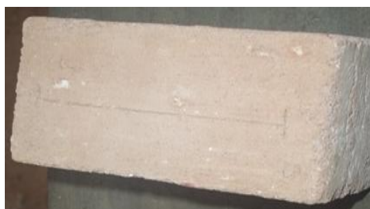
Fig. 2. The linear shrinkage of the bricks
