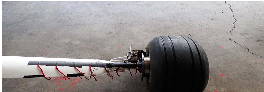
Figure 3. Instrumentation and telltale's record attitude and airspeed.
