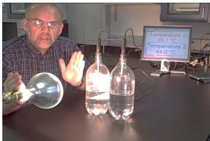
Fig. 20. Carbon dioxide experiment proves excess heat trapping – nine degrees C hotter [52]
