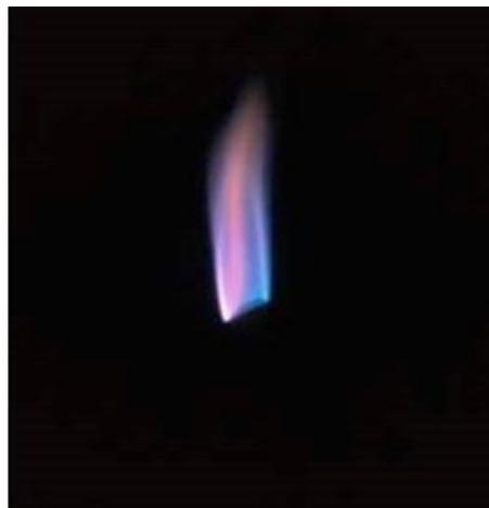
Fig. 13. Biogas burning with a blue flame
