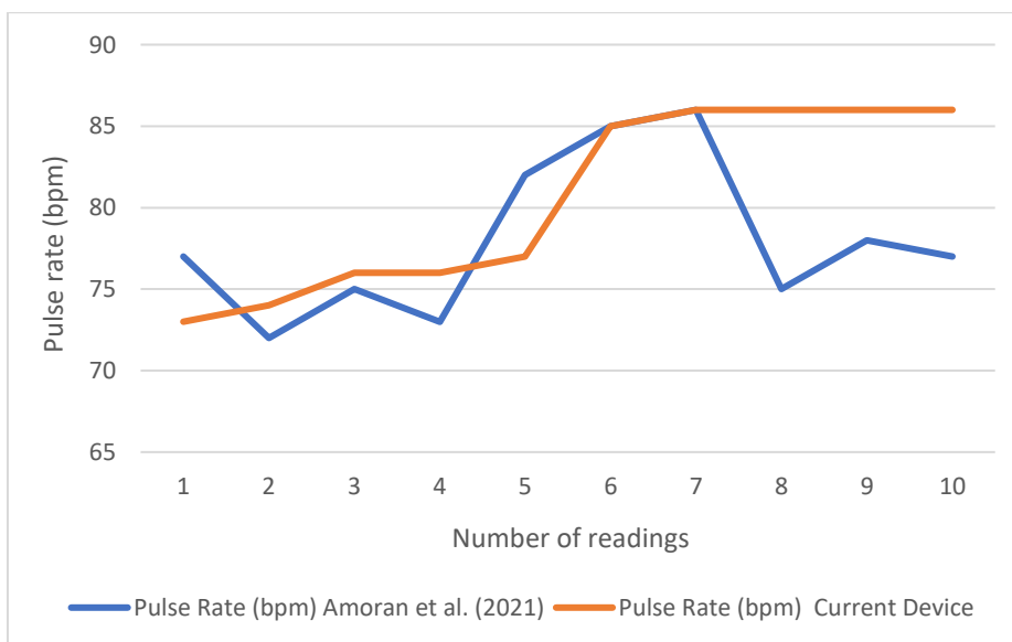
Fig. 21. Comparison of device pulse rate reading with previous work
