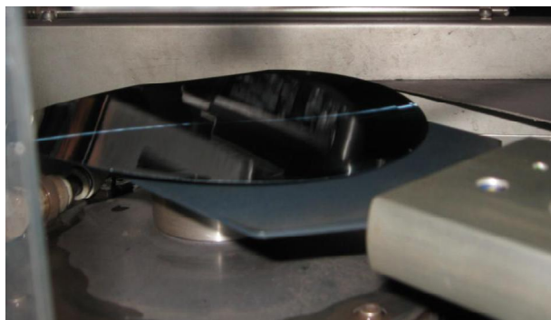
Fig. 6. Vacuum error on the robot arm
