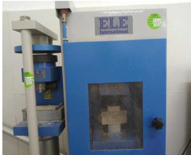
Fig. 4. The bending and compression testing equipment
